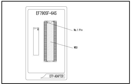
Fig. 2.1 Insertion Direction of MCU
